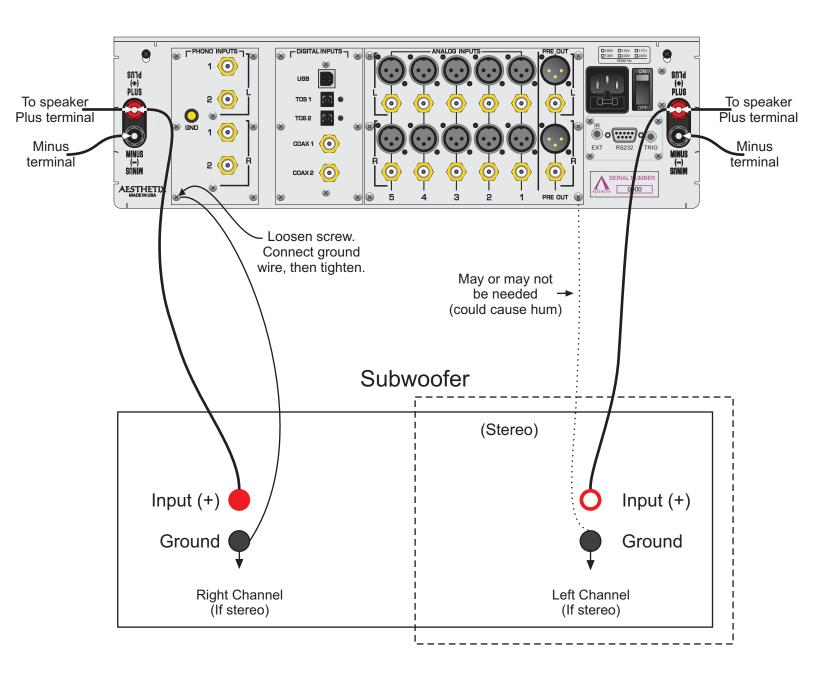
**WARNING**: Never connect the minus (-) speaker output of a Mimas to Ground. Damage to the Mimas and / or the sub could result.
